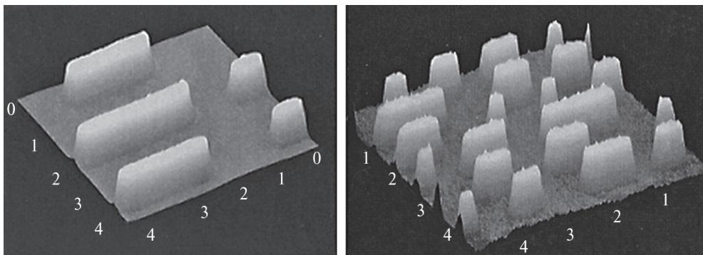
**Fig. 5.34.** Information recording area with different recording density: CD format (track pitch of  $1.6\mu\text{m}$ ) (a); DVD format (track pitch of  $0.74\mu\text{m}$ ) (b)
