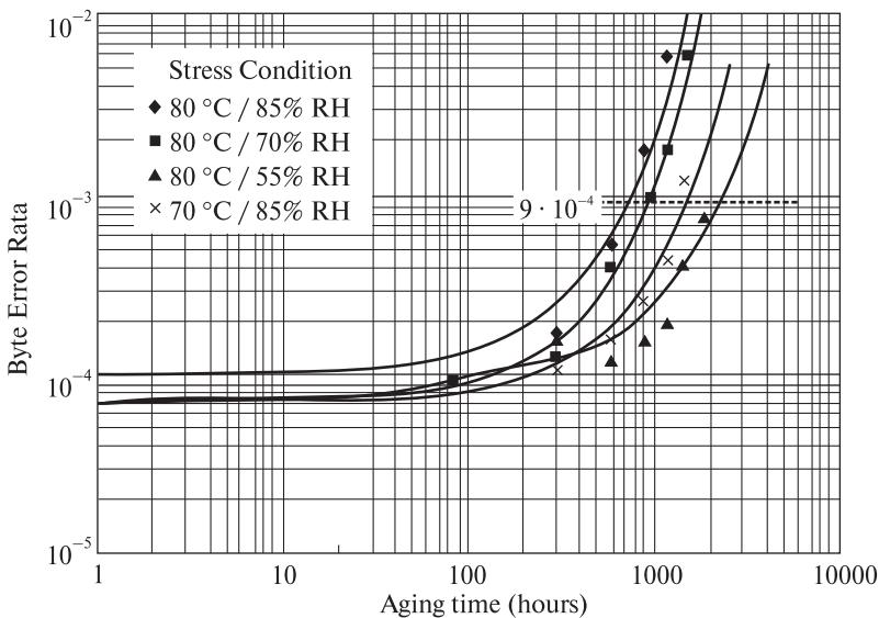
**Fig. 6.2.** Typical experimental result of BER measurement [144]
