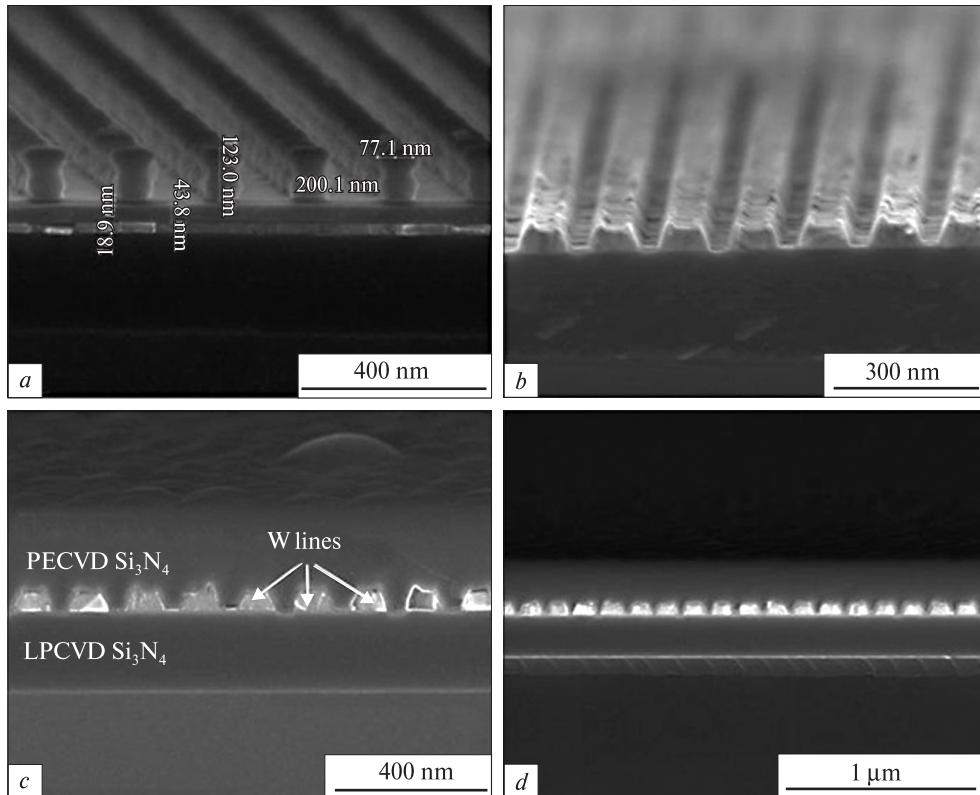
**Fig. 5.11.** Scanning electron micrograph of the test sample before etching (a). Scanning electron micrograph of the test sample after etching containing W lines (b). Scanning electron micrograph of the cross-section of the encapsulated lines in the test sample (c), scanning electron micrograph of the sample after 1 h. at 473 K [99] (d)
