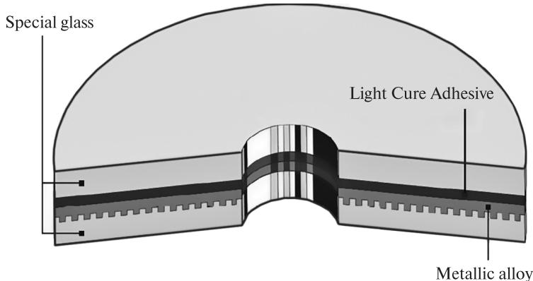
**Fig. 5.5.** Glass disc for long-term data storage [98]
