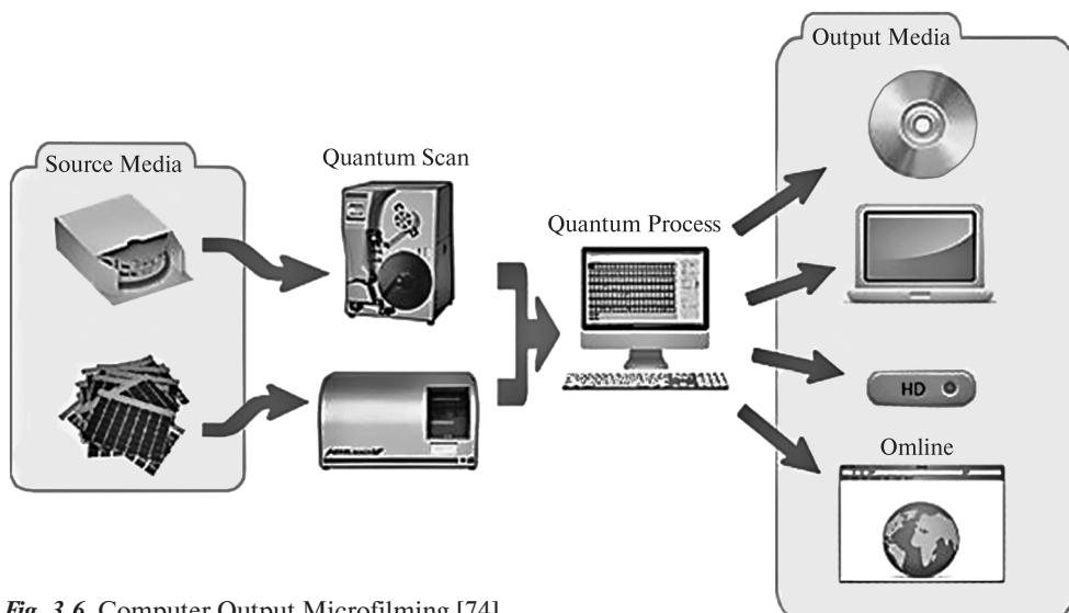
**Fig. 3.6.** Computer Output Microfilming [74]
