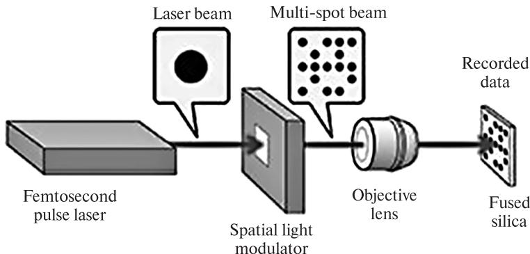
**Fig. 5.15.** The concept of storing data optically in the bulk of non-photosensitive transparent materials [162]
