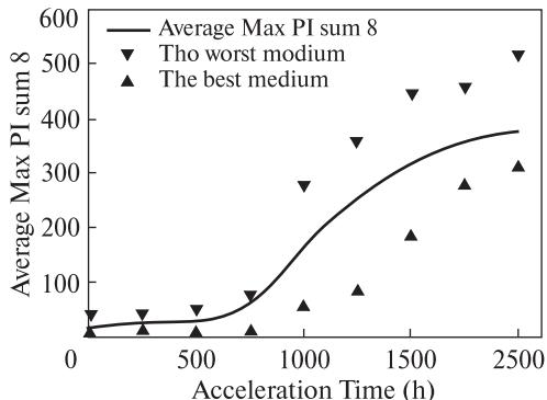
Fig. 6.8. Average max PI sum 8 value with aging time. The PI sum 8 values were averaged from 20 DVD + R test disks [137]
