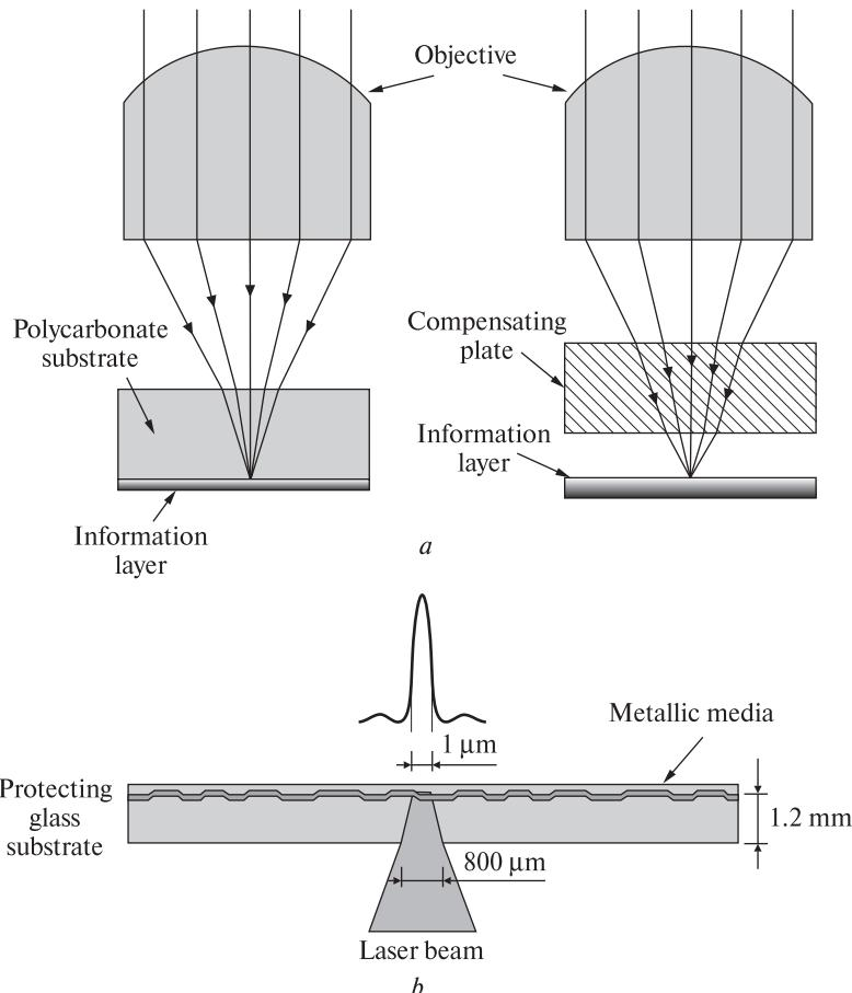
**Fig. 5.33.** Modification of optical system for information read-out from metallic media (a); metallic media with protecting glass substrate (b)
