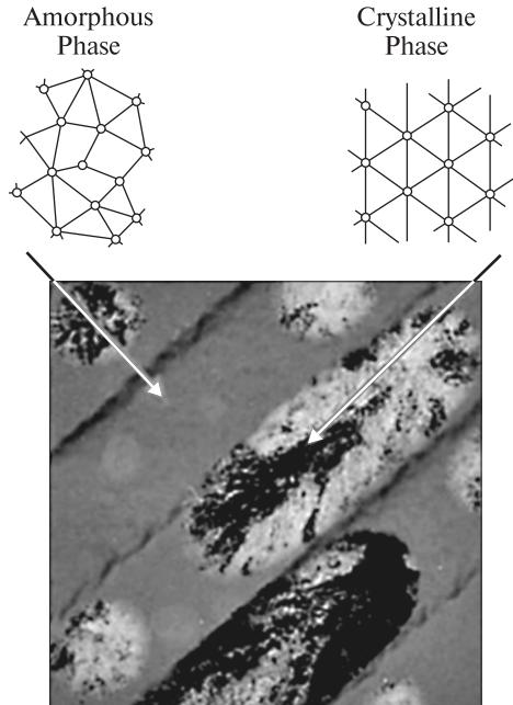
Fig. 5.3. Bits of Phase Change UDO disk [98]
