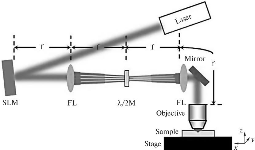
**Fig. 5.17.** 5D optical storage writing setup: femtosecond laser, spatial light modulator (SLM), Fourier lens (FL), half-wave plate matrix ( $\lambda/2$  M), dichroic mirror, 1.2 NA water immersion objective, silica glass sample, translation stage [163]
