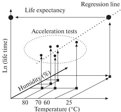
**Fig. 6.1.** Outline of the acceleration Eyring model [157]
