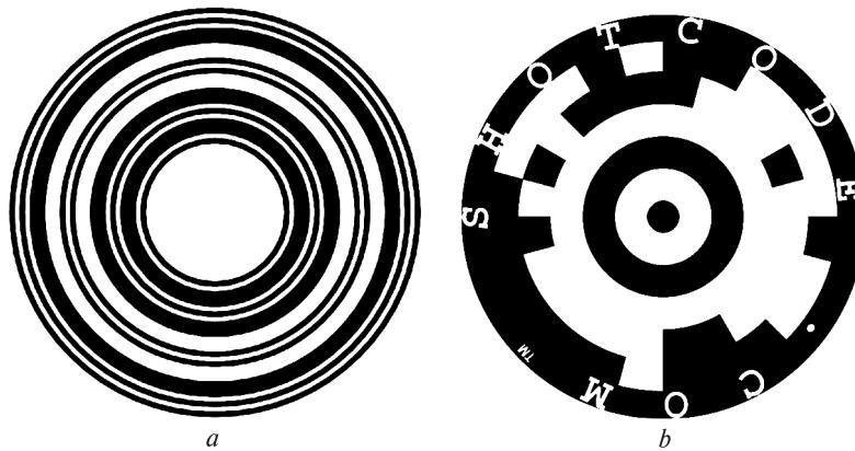
Fig. 2.2. Circular barcode structure: *a* — Circular 1D barcode, *b* — ShotCode
