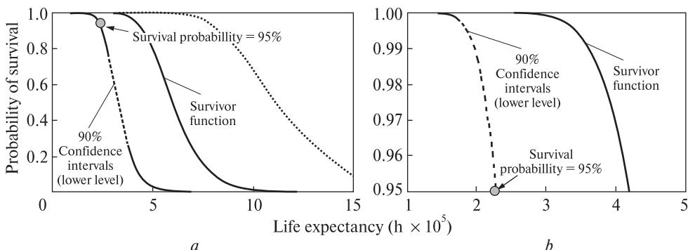
**Fig. 6.6.** Probability-of-survival function at 25 °C / 50%RH (a), expanded scale (b)
