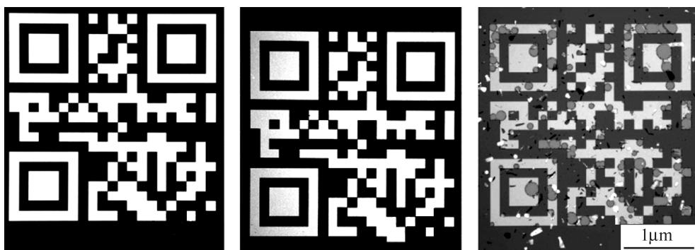
**Fig. 5.13.** Optical microscope images of the same QR code; left — after fabrication, center — after 2 hours at 613 K and right — 2 hours at 763 K [115]
