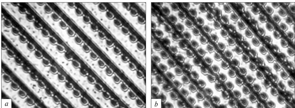
**Fig. 4.8.** External appearance of the recording zone on the optical carrier: data recording is carried out from one side of a guide track (a) and from both sides (b)
