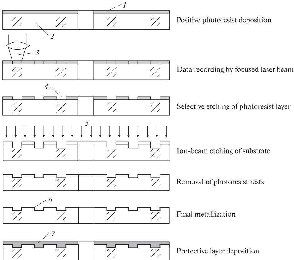
**Fig. 5.6.** Scheme of data recording process on the optical disc for long-term data storage: 1 — sapphire substrate; 2 — Cr film; 3 — positive photoresist layer; 4 — focused laser beam; 5 — etching mask; 6 — ion beam; 7 — reflective metallic layer [92]
