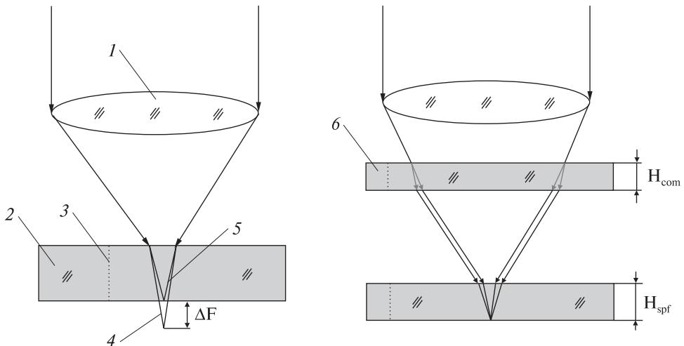
**Fig. 5.26.** Schematic representation of aberration compensation: 1 — objective lens, 2 — sapphire substrate, 3 — optical axis, 4 — extraordinary ray, 5 — ordinary ray, 6 — compensating plate
