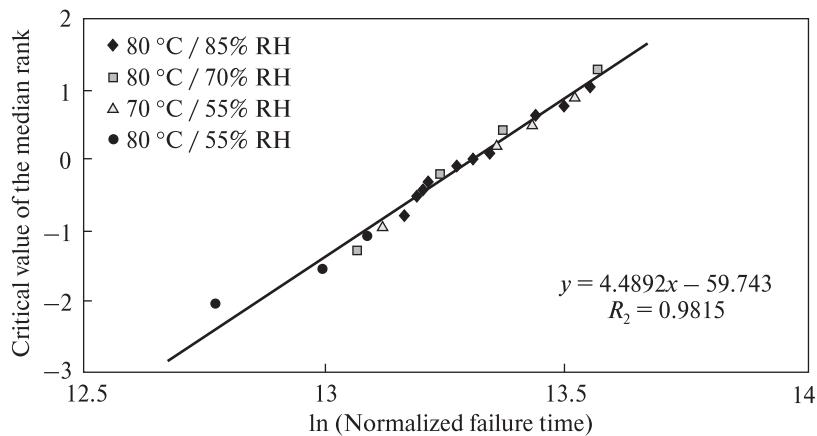
**Fig. 6.5.** Combined life time data normalized to 25 °C / 50% RH [84]
