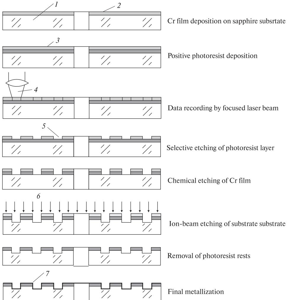
**Fig. 5.28.** Improved scheme of data recording process on the optical disc for long-term data storage: 1 — sapphire substrate; 2 — Cr film; 3 — positive photoresist layer; 4 — focused laser beam; 5 — etching mask, 6 — ion beam, 7 — reflective metallic layer
