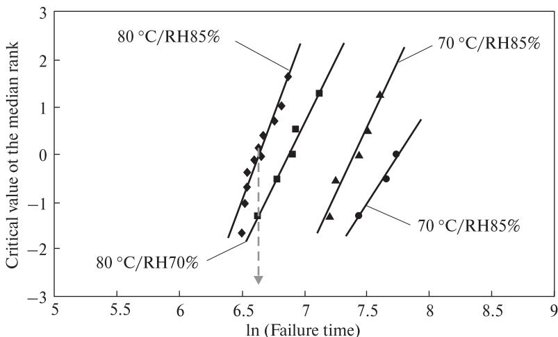
**Fig. 6.3.** Relation between the limit value of  $F(t)$  for the median rank of lifetime data and the natural logarithm of the lifetime data [94]
