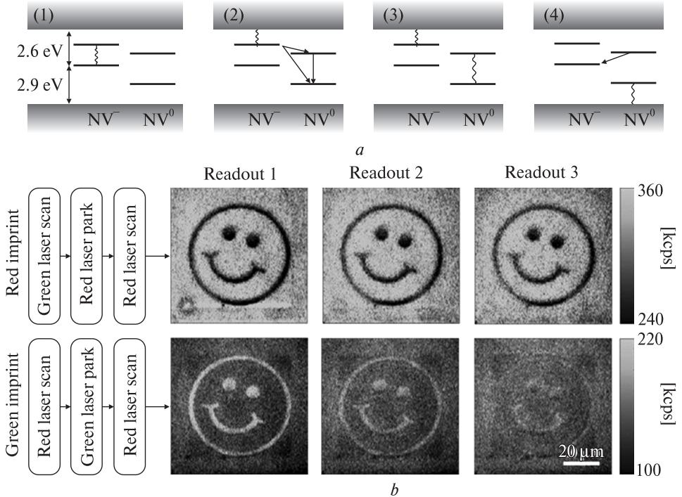
**Fig. 5.18.** Charge manipulation and readout in diamond
