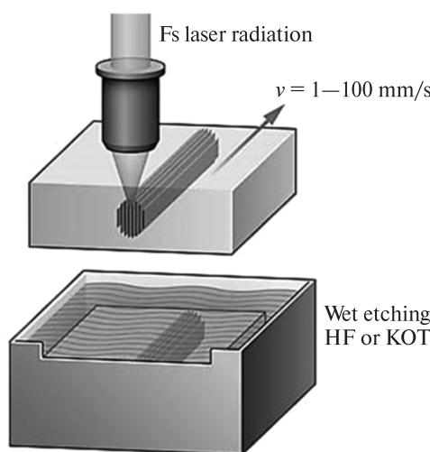
**Fig. 5.22.** Processing steps of ISLE: Writing of the modification with fs-laser radiation and subsequent selective wet chemical etching of the modified material
