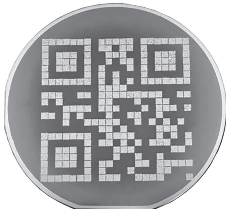
**Fig. 5.12.** Design of the HDP disk. Each pixel in the large QR codes consists of a micro-QR code [114]
