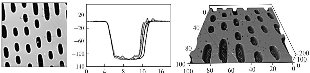
*Fig. 5.29.* AFM image of sapphire substrate after ion-beam etching
