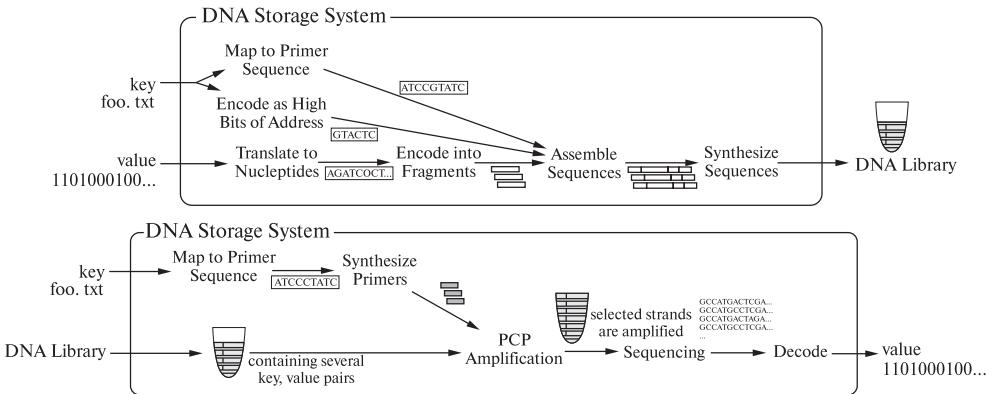
**Fig. 3.9.** Overview of a DNA storage system [81]
