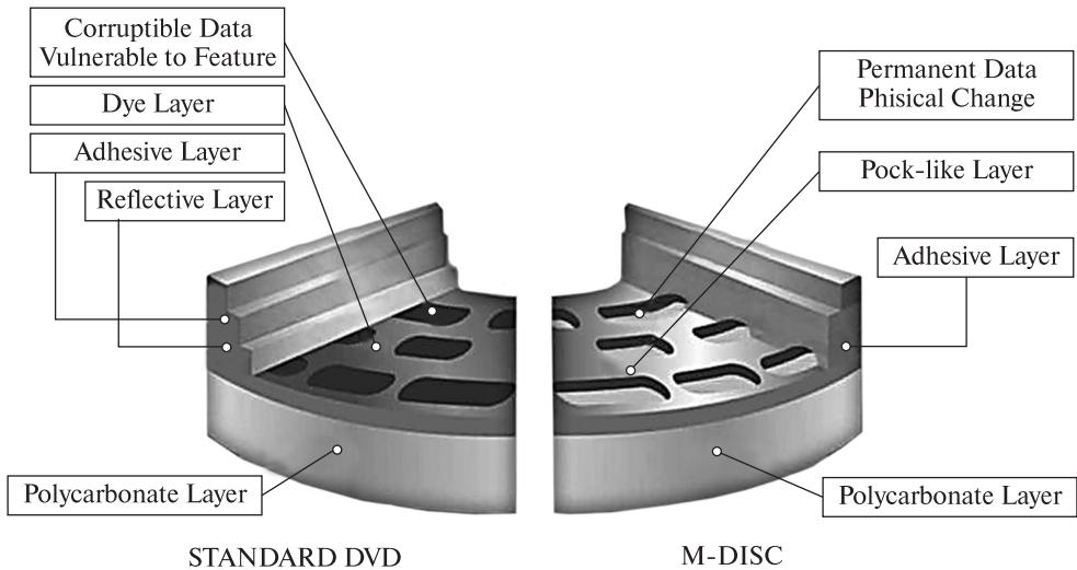
**Fig. 5.4.** Structure comparison of standard DVD and M-Disc [98]
