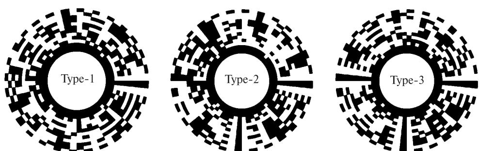
**Fig. 2.4.** Three types of generic circular 2D barcodes [39]
