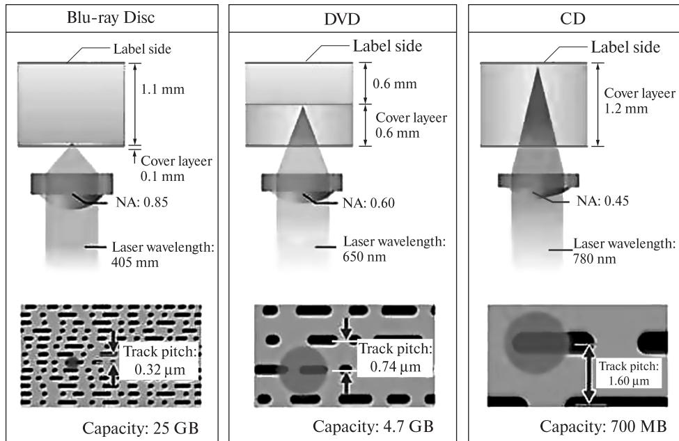
**Fig. 4.1.** Improving the systems of optical information recording [89]
