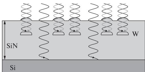
**Fig. 5.9.** W- $\text{Si}_3\text{N}_4$  WORM medium, which is readable by constructive interference on the silicon base and destructive interference on the tungsten islands [107]
