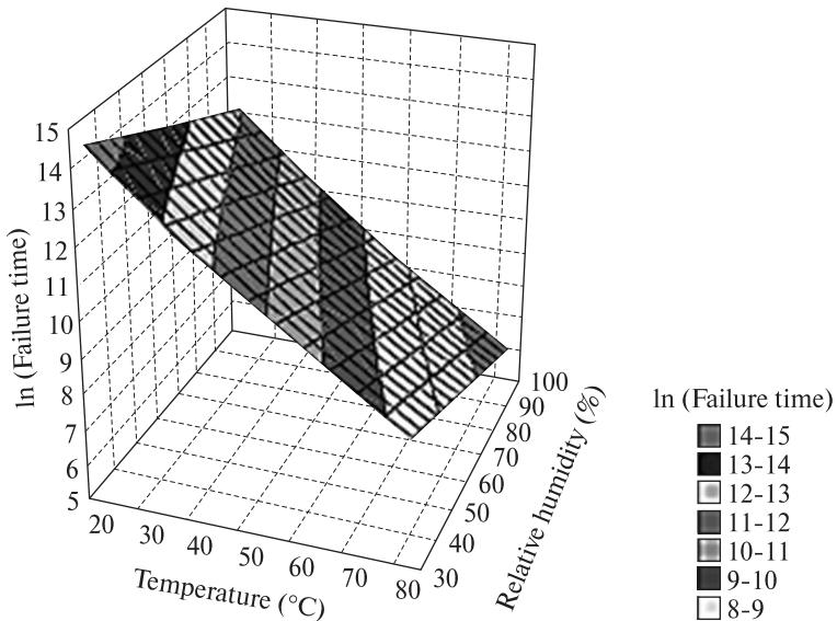
**Fig. 6.4.** Natural logarithm of failure time (log mean) at temperature range 20 °C-80 °C and RH range 30%-100% [84]
