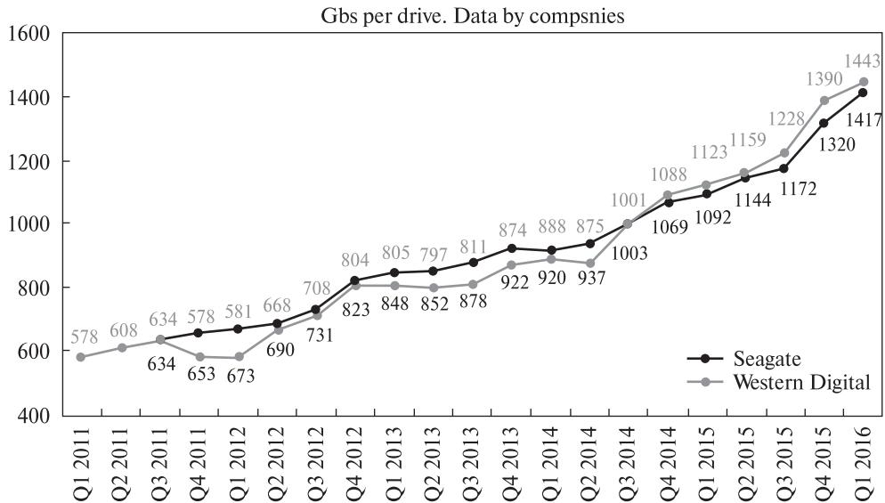
Fig. 3.1. Increase in areal density on hard magnetic disks [52]
