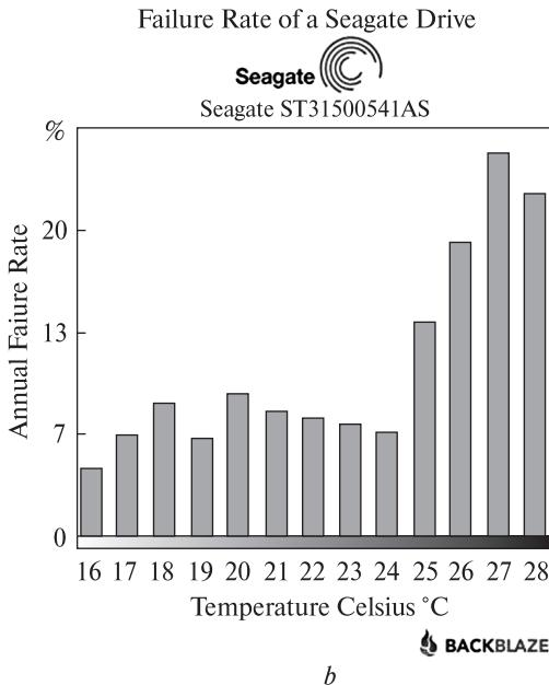
**Fig. 3.2.** Hard drive failure rate as a function of time and temperature [53]
