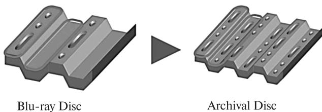
Fig. 4.4. High-Capacity Land/Groove Recording [183]
