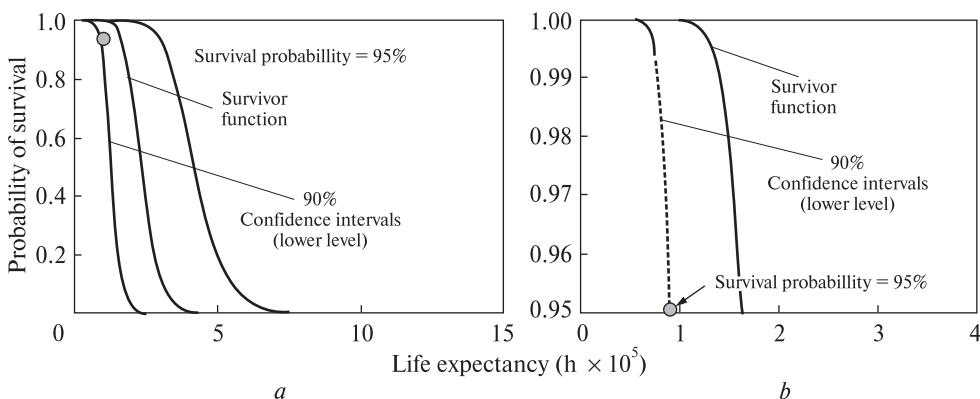
**Fig. 6.7.** Probability-of-survival function at 30 °C / 60%RH (a), expanded scale (b)
