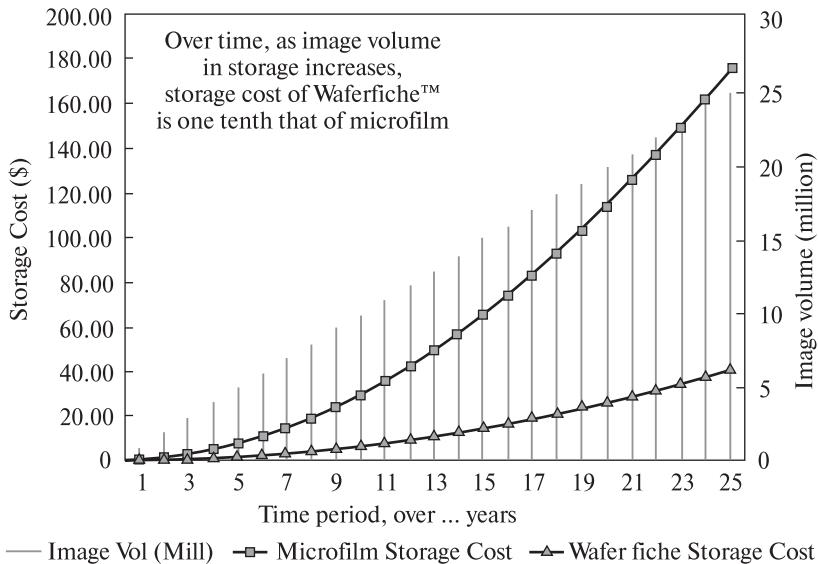
Fig. 5.7. Comparison of storage costs – microfilm and waferfitche [111]
