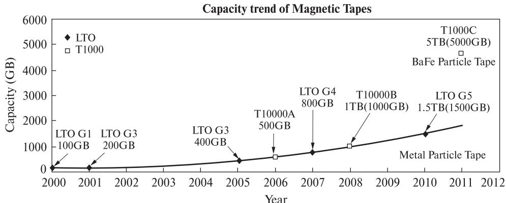
**Fig. 3.3.** Increasing the capacity of magnetic tapes [61]
