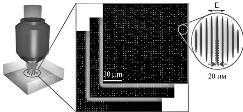
**Fig. 5.16.** 5D optical data storage, written in fused quartz using a femtosecond laser. Three spatial dimensions and two optical ones (the slow-axis orientation and the retardance) are exploited. Each voxel contains a self-assembled nanograting which is oriented in a direction perpendicular to the light polarization [163]
