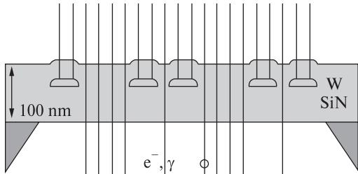
**Fig. 5.8.** W- $\text{Si}_3\text{N}_4$  WORM medium, which is transparent to electron or photon beams [106]
