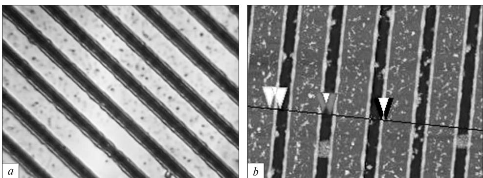
**Fig. 4.9.** Guide tracks on the optical disc carrier with  $\text{Te}_{14}\text{Sb}_{10}\text{Se}_{61}\text{Ge}_{15}$  recording medium (track pitch is  $1.6 \mu\text{m}$ ). The images are obtained using: a — optical microscope; b — scanning tunnel microscope [183]
